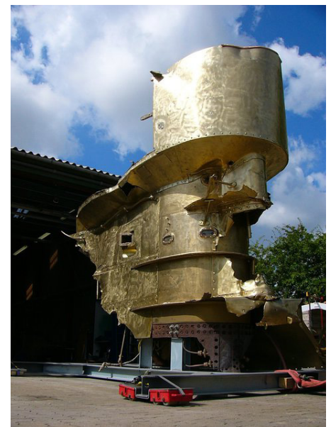
Above: Painting by Johannes E. Møller depicting Four German mine trawlers being fired on and were later sunk by British Naval forces on the west coast of Jutland. Below: the 11-ton conning tower from the British submarine E-50 which is on display with kind permission of the Royal Navy. On 31 January 1916 the E-50 struck a mine, and the whole crew of 30 was lost. In the museum they are remembered with a memorial plaque.
